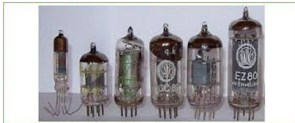
Electrons will flow from the filament to the plate when the plate is positive, but not when it is negative.
